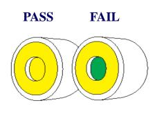
This is a Go/No Go test, the result should be either Pass or Fail as shown above. It should not be used in an attempt to quantify water levels but a slight intermediate colour change can indicate a trace of water in the product somewhere between 0 and 30ppm, and this is shown in the records as Trace if required by local regulations.
